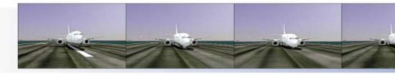
derotation should be performed so that the flight crew immediately starts flying the nosewheels smoothly onto the runway when the main wheels touch down. Flight crews can accomplish this by controlling the airplane pitch rate while
